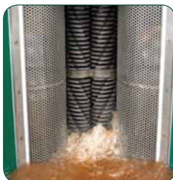
A model CDD4020-XDS2.0 with optional perf drums.
