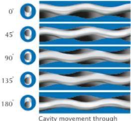
Cavity movement through 180° of Rotor rotation
