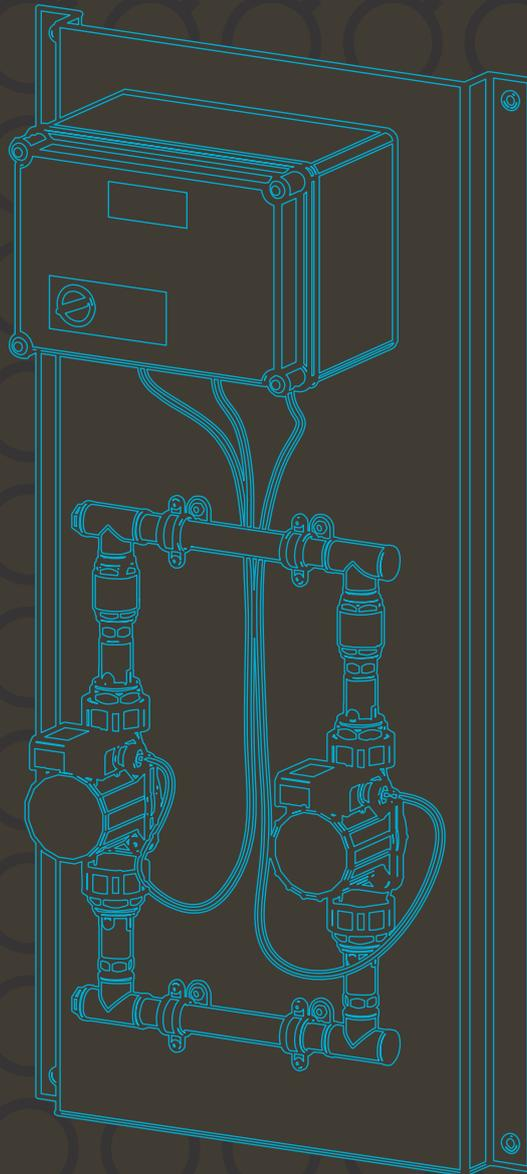
**The e-Boost Packaged Hot Water Circulation Systems are automated twin pump circulation packages designed to reduce energy consumption and ensure consistent hot water supply.**
