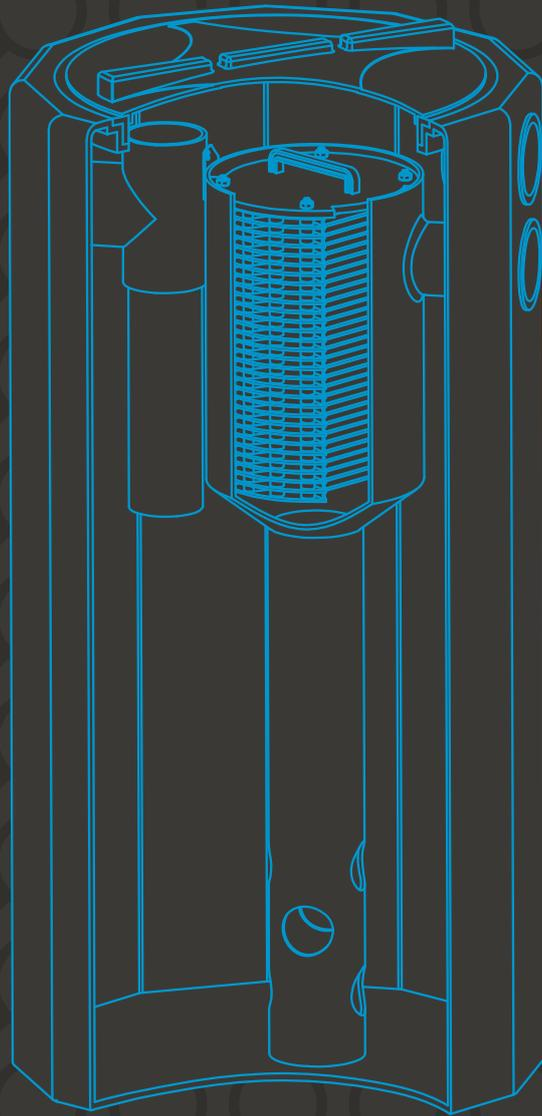
**The compact Grease Muncher GM700 reduces installation and maintenance costs compared with traditional large concrete arrestors. The option for above-ground mounting allows for flexibility and portability of installation and relocation.**
